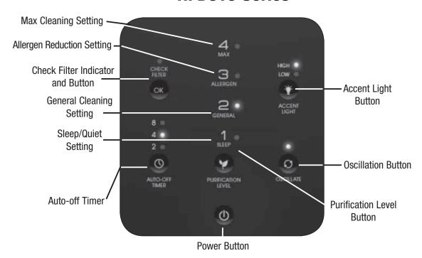
**Check Filters Button** – When it is time to check and clean the filter, an indicator light will illuminate. When this light comes on, you will need to clean your primary ifD<sup>®</sup> filter and clean or replace your pre-filter. (See Filter Cleaning instructions on page 10). After you have cleaned or replaced the filters, press and hold the Check Filters button for approximately 2 seconds until the light goes off.
